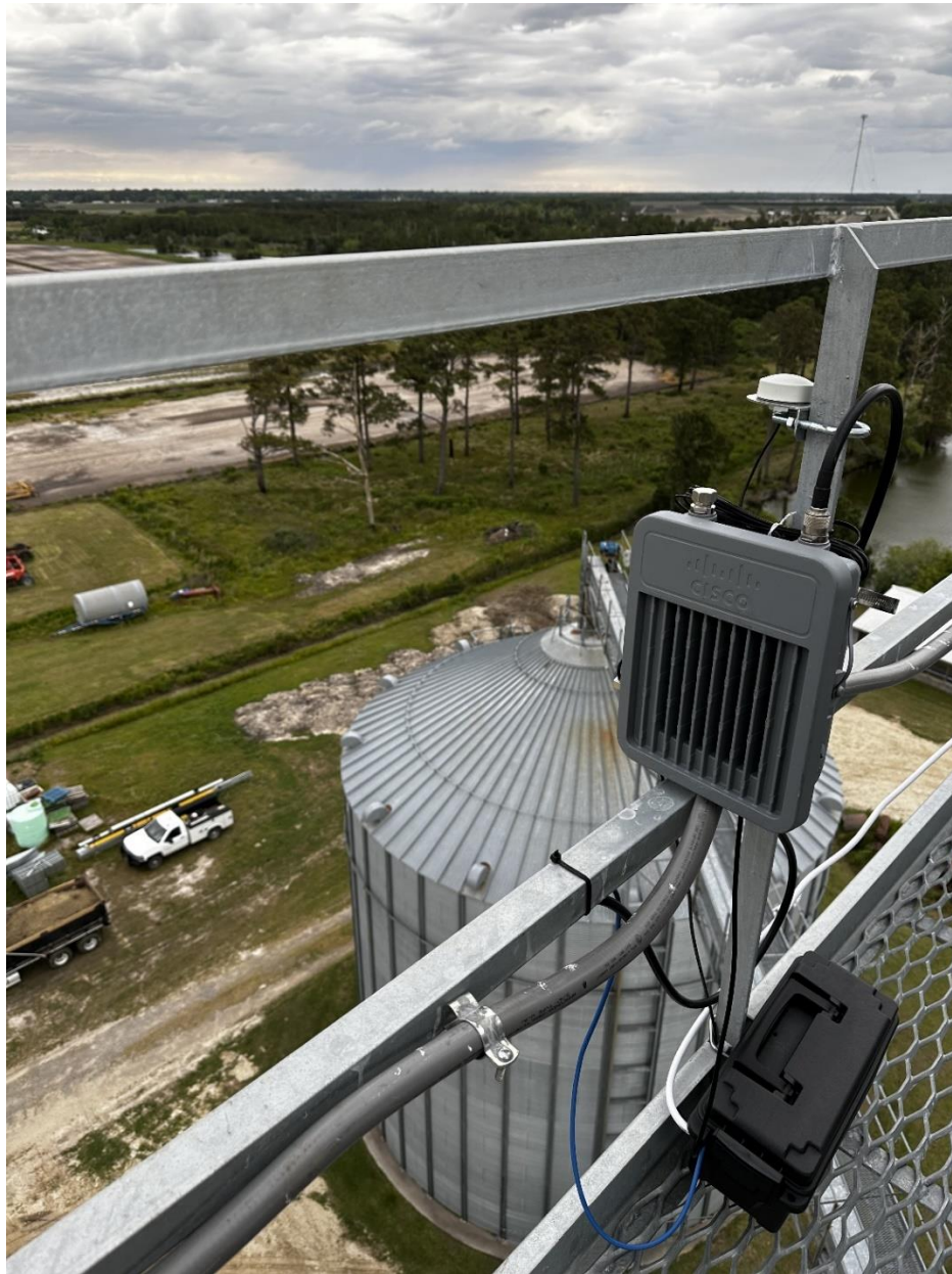
Figure 2, LoRaWAN gateway deployed on the premises of the farm.
