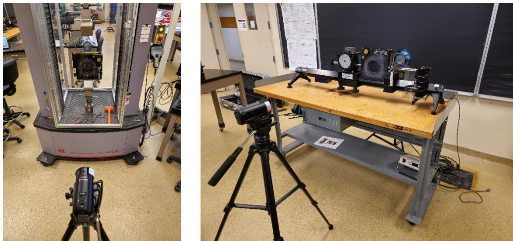
(a) (b) Figure 7: Photoelasticity setup: (a) Tension tests; (b) Torsion tests.
