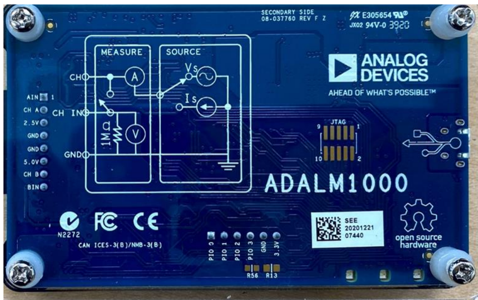
Figure 4: ADALM 1000 Analog Device
