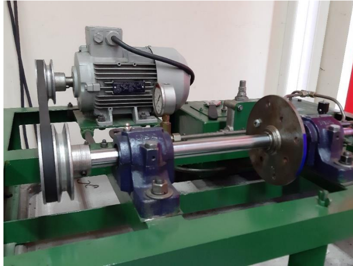
Figure 1 Laboratory Rotor Test Rig for Single-Plane Balancing Experiments at Universidad Austral de Chile
