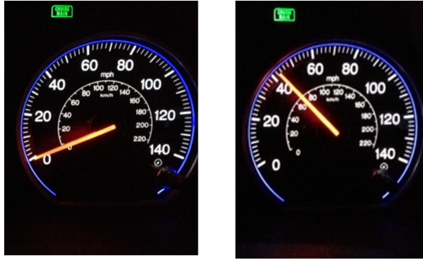
Figure 14: Using speedometer to calculate the total distance traveled on straight highway
