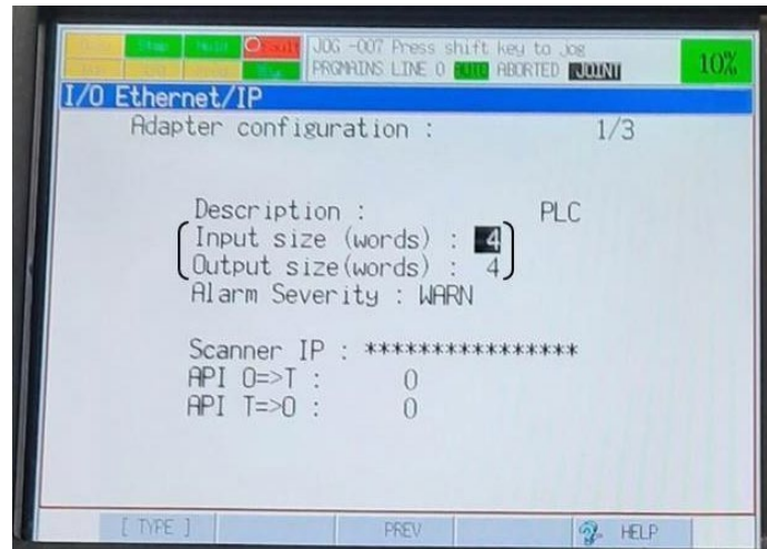
Figure 10. Communication protocol settings on the robot teach pendant
