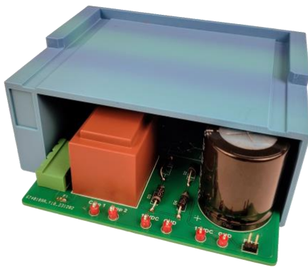
Figure 7. Protective housing and work tray with custom PCBA (prototype).
