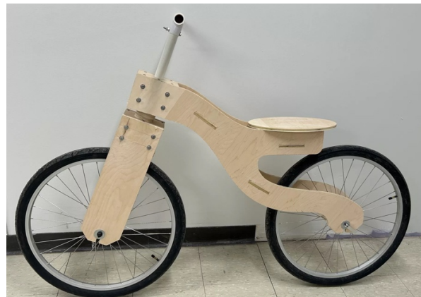
Figure 2. Example student work for final bike frame design: CAD assembly drawing (left) and assembled prototype (right).
