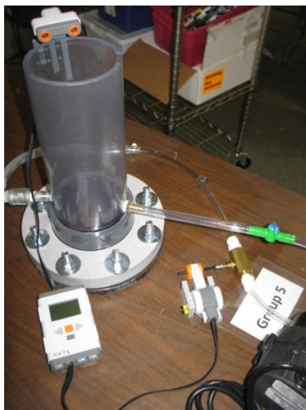
144 Figure 1. Tank level control using LEGO NXT robotics components [35].
