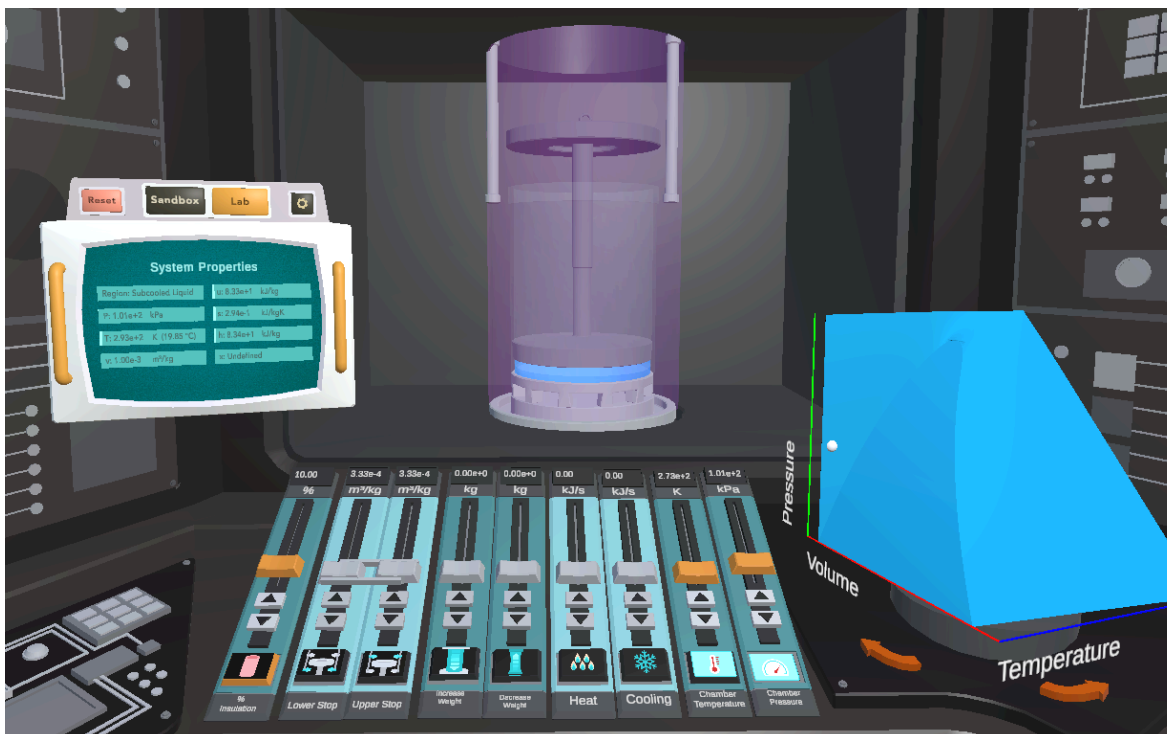
Figure 2: Image of a prototype for ThermoVR version 2, with the tablet device on the far left, a piston-cylinder apparatus in the top middle, controls in the bottom center, and the 3d thermodynamic graph on the lower right
