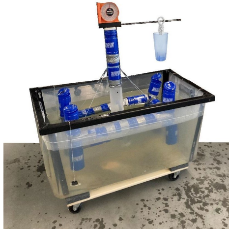
Figure 1. The test tank including a student-designed platform. Note the reinforcing collar that attaches to the mooring chains and supports ~400 lbs of water. A weight is put into the cup some distance from the top of the tower to apply a moment.
