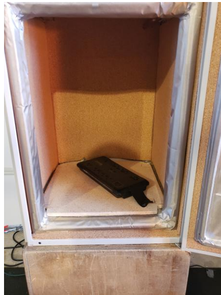
Figure 10: Second Layer of Cork for the Cabinet's Interior
