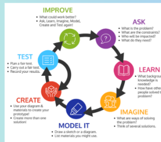
Engineering design cycle Adapted from Purdue's rollercoaster challenge
