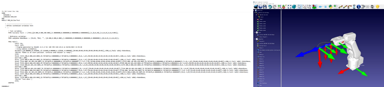
Figure 5. a) Sample Ballbar setup and measurement program (left) generated by Robodk. b) Robodk tool path simulation for ABB IRAB 120 robot.
