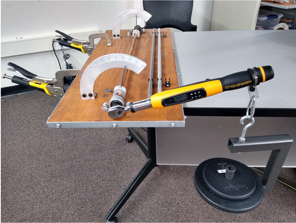
Figure 3: As-Built Custom Torsion-Testing Machine
