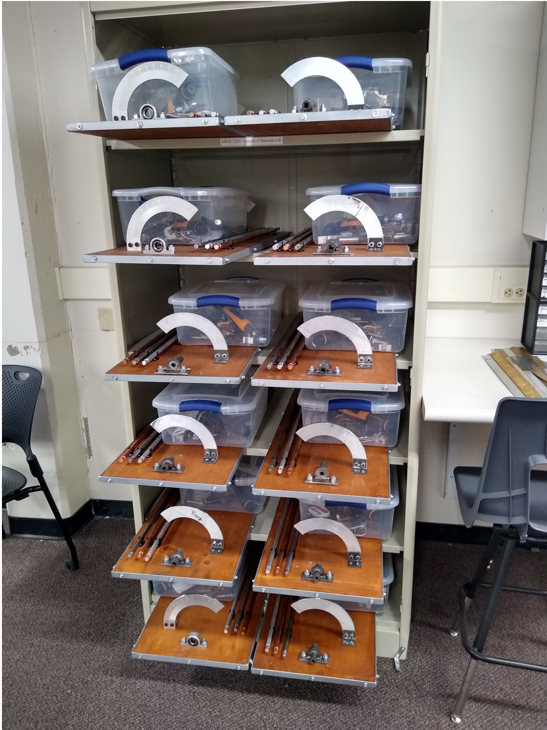
Figure 4: Cabinet with 12 custom torsion-testing machines
