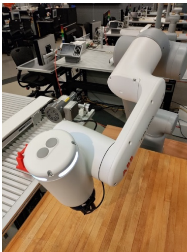
Fig. 3. Buttons located at “head” of CRB.
