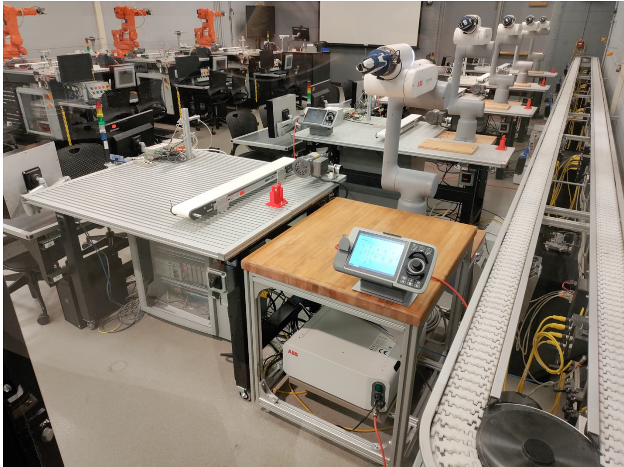
Fig. 5. Mobile CRB in “split” rolling workstation.
