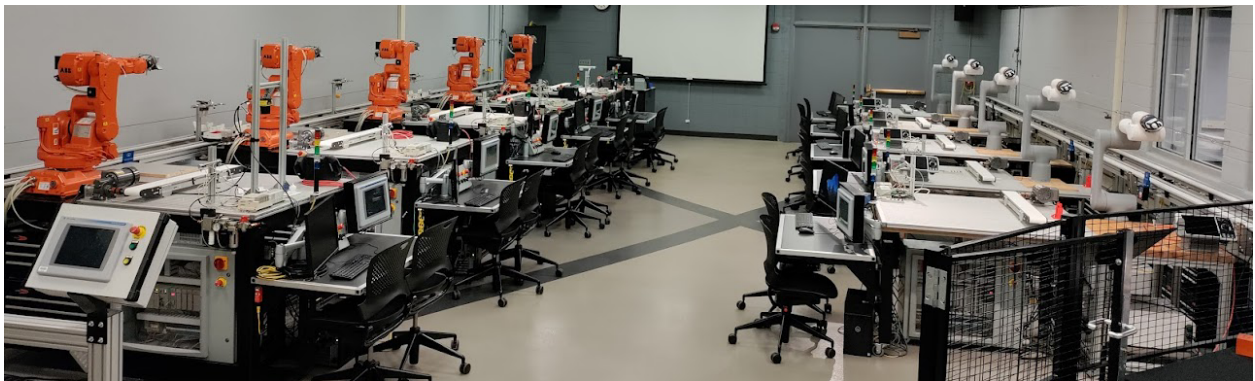
Fig. 2. New IML layout. (Left) Five IRBs with original workstation layout. (Right) Five CRBs with the redeveloped design.
