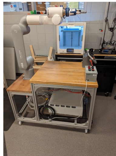
Fig. 4. CRB mobile cart in machine tending application.
