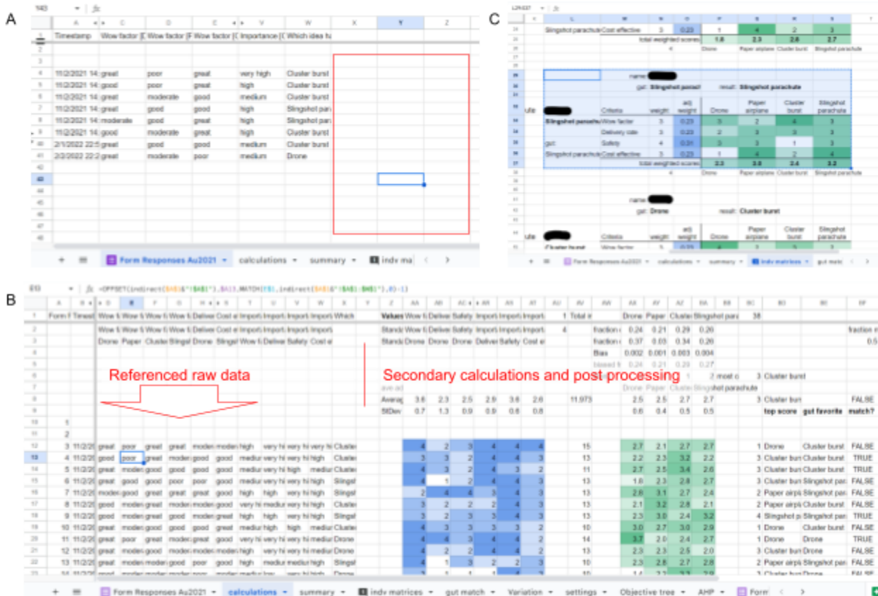
Figure 2: A) Responses from a Google Form can be output into Google Sheets, but setting up post-processing equations in the columns to the right (red box) would result in them being overwritten with blank cells when new results are submitted. B) Instead, results can be referenced from a separate spreadsheet tab (here, using the equation “=OFFSET(indirect($A$1&"!$A$1"),$A13,MATCH(E$1,indirect($A$1&"!$A$1:$W$1"),0)-1)”, ordered in a way that is more intuitive, and additional calculations can be run. C) The calculated results can be organized into tables, formatted, and copied into Google Slides as a “linked object.”
