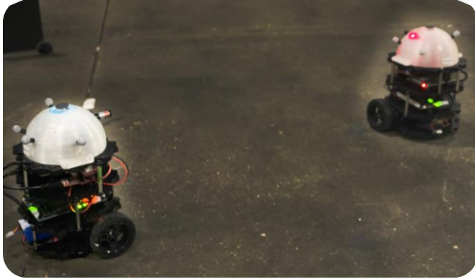
Fig 3. Physical Turtlebots for swarm testing, with mounted laser tag receivers.
