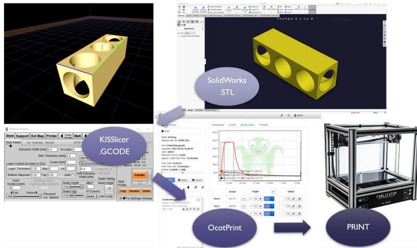
Figure 3: Remotely 3D Printing FDM process via OctoPrint.
