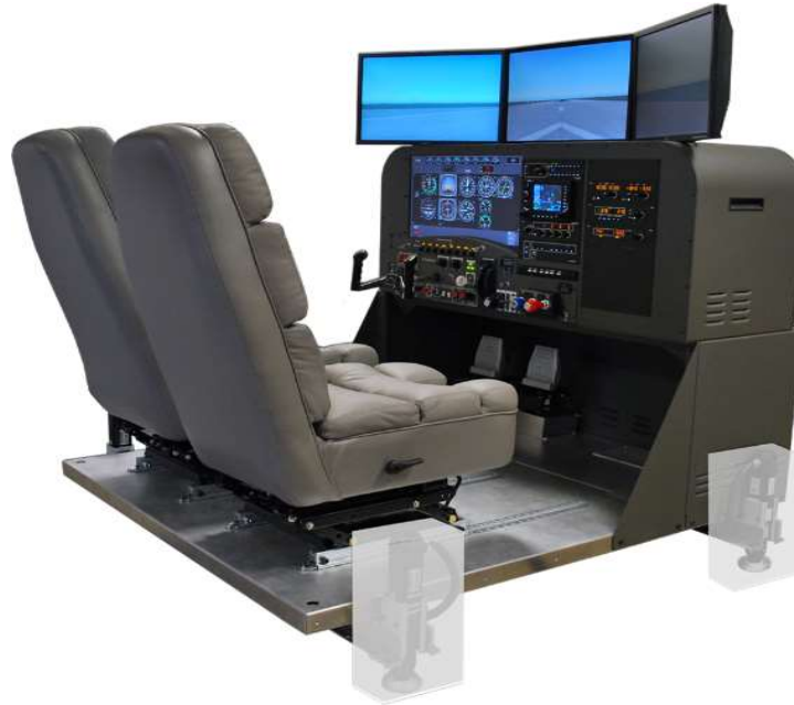
Figure 2: Flight Training Device (FTD) - aka Flight Simulator
