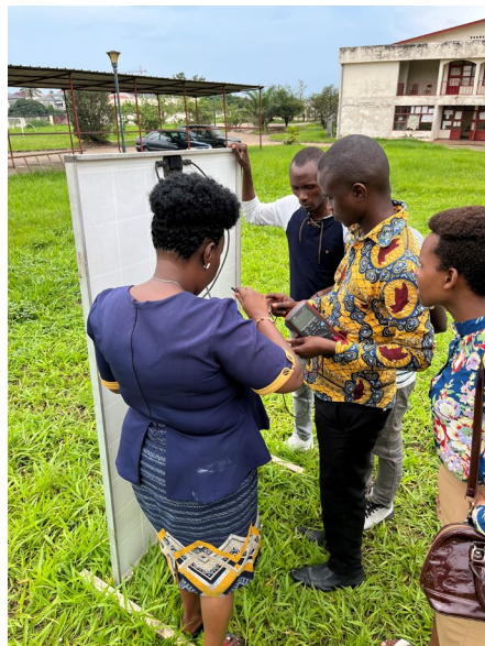
Figure 1. Professors and students at ENS characterizing a solar panel
