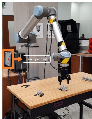
(a) The physical UR10 industrial robot arm with one of the three aluminum blocks (far-right) already placed at the drop off location
