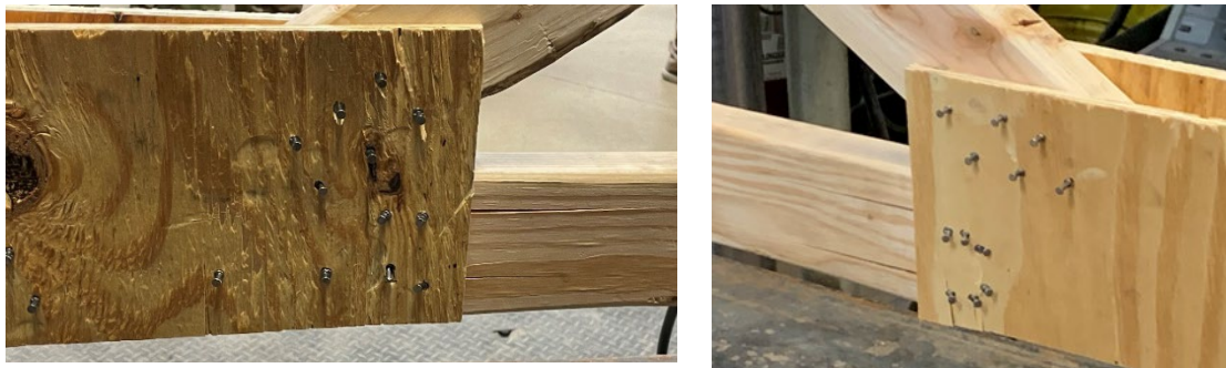
Figure 8: Shear deformation of duplex nails and axial failure of tension members during experimental testing.
