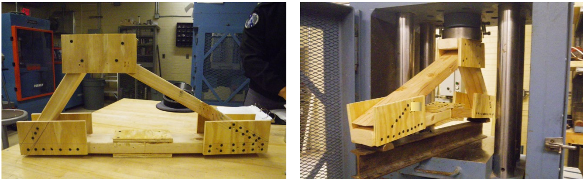
Figure 6: Subproject truss construction and testing
