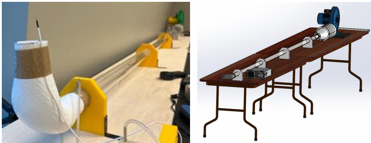
Figure 3. Experimental setup and SOLIDWORKS model for measurements of pressure drop.
