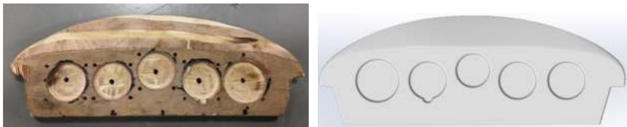
Figure 2a) Instrument panel pattern made of wood and shown as a SOLIDWORKS model
