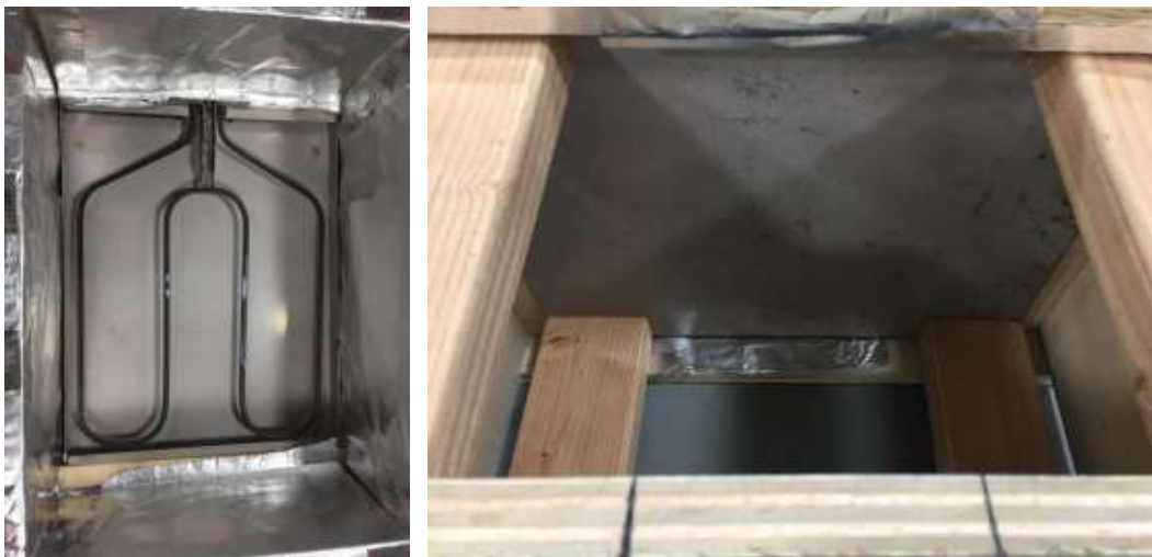
Figure 3b) Heating element Figure 3c) View from below of sheet metal pan
