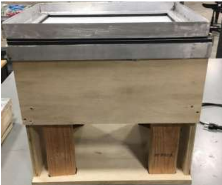
Figure 4b) Aluminum frame mounted on top of heating unit
