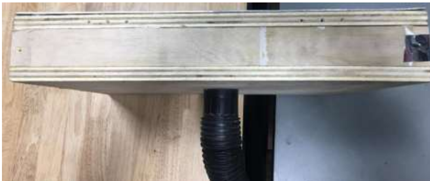
Figure 5b) Side view of vacuum hose attachment to suction box
