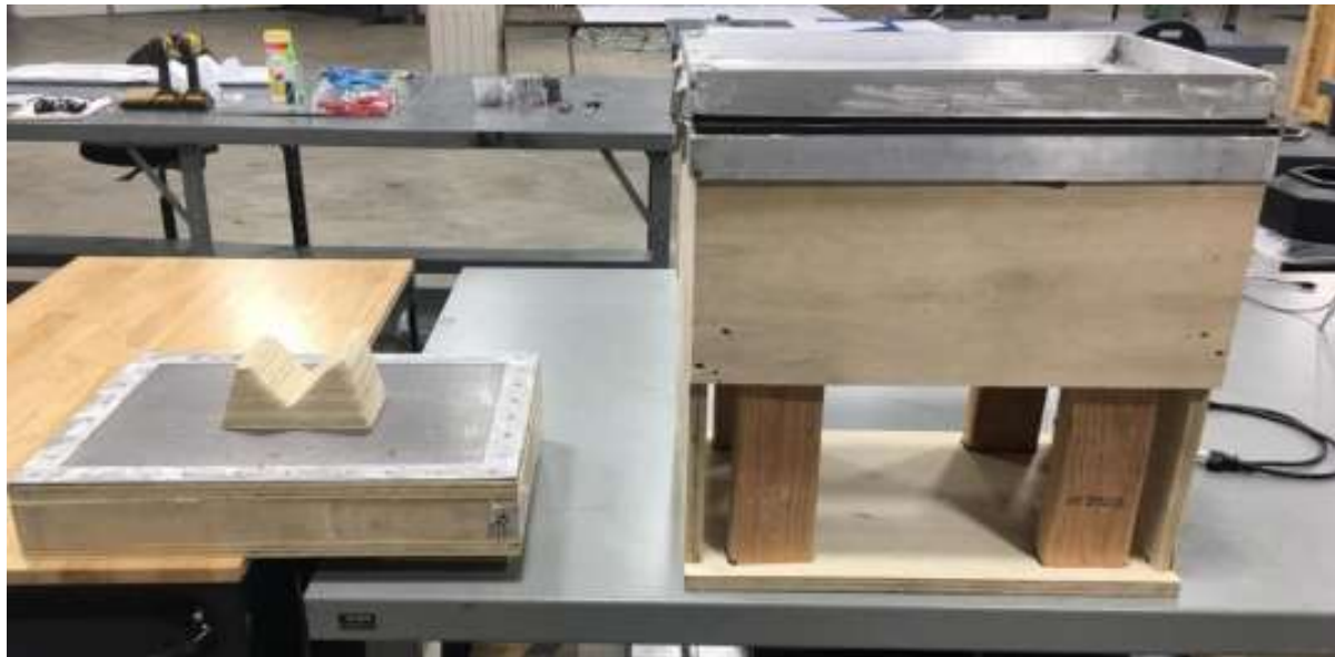
Figure 6a) Heating unit with aluminum frame and suction box with mold pattern side by side.
