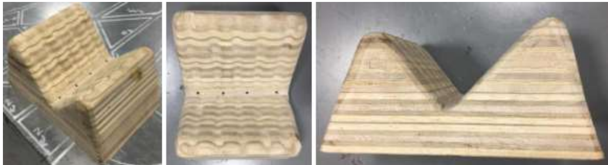
Figure 2b) Seat pattern made of plywood
