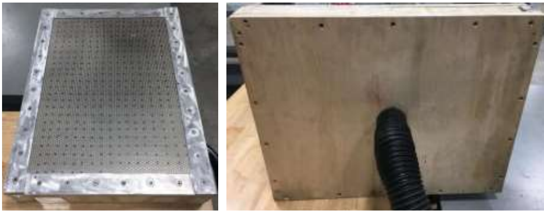
Figure 5a) Suction box for thermoforming
