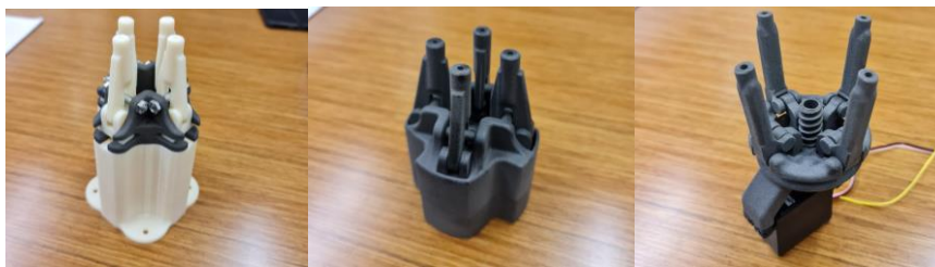
Figure 12: 3D printing of different design iterations of the origami, final to the right
