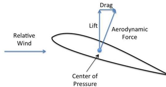
**Figure 2.** The Visualization of Lift and Drag Forces on an Airfoil
