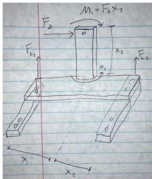
**Figure 4.** Statics Diagram for Drag Moment Adjustment
