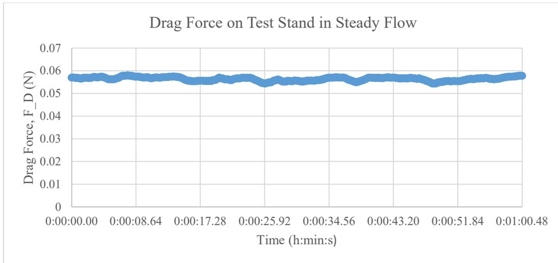
**Figure 15.** Drag Force on Test Stand over Time
