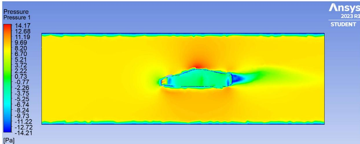
**Figure 10.** Pressure Profile on Corvette C8
