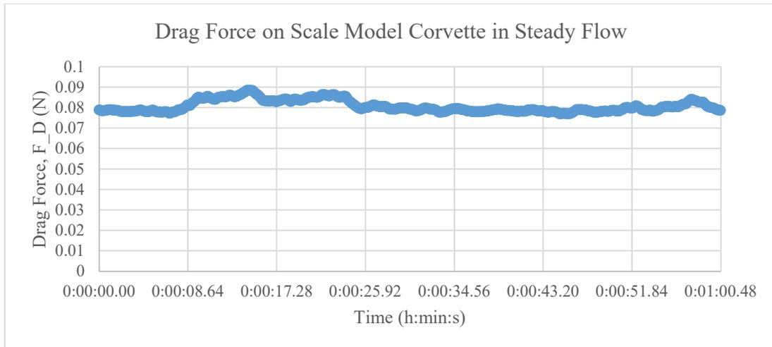
**Figure 13.** The Drag Force on a Scale Model Corvette over Time
