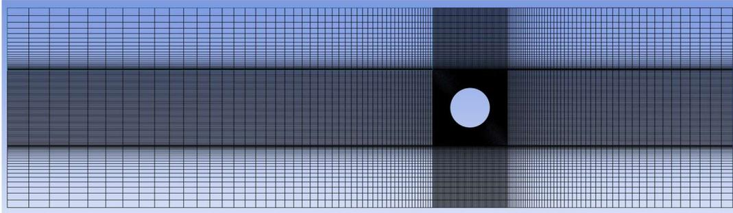
**Figure 7.** Bias Meshing around Cylinder to Increase Simulation Accuracy
