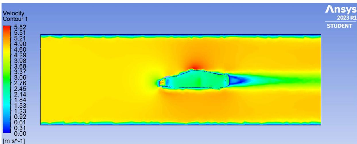
**Figure 9.** Velocity Profile on Corvette C8
