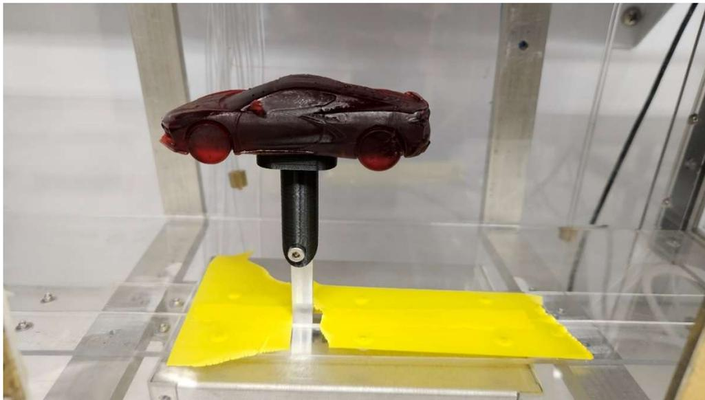
**Figure 12.** The Scale Model Corvette Mounted in the Wind Tunnel.
