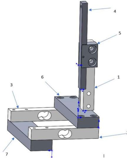
**Figure 3.** The Design of the Force Balance System
