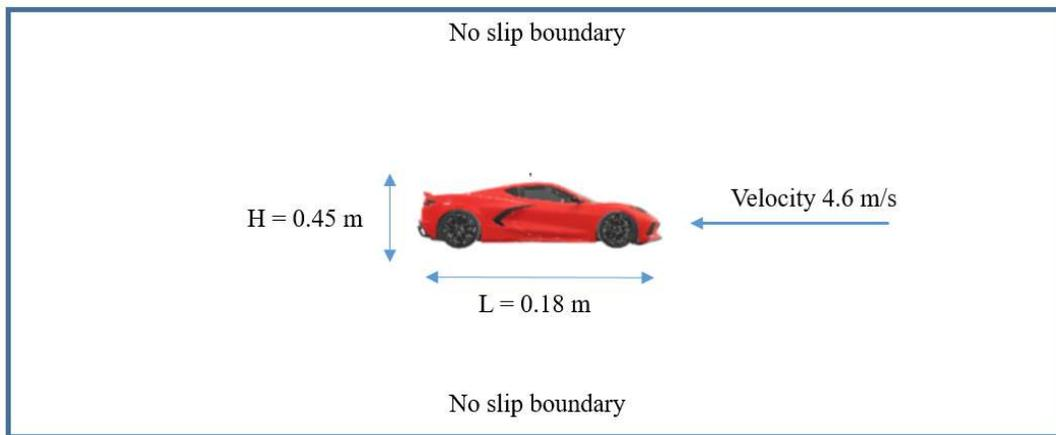
**Figure 6.** The Physical Model of the Corvette Car Model [6]
