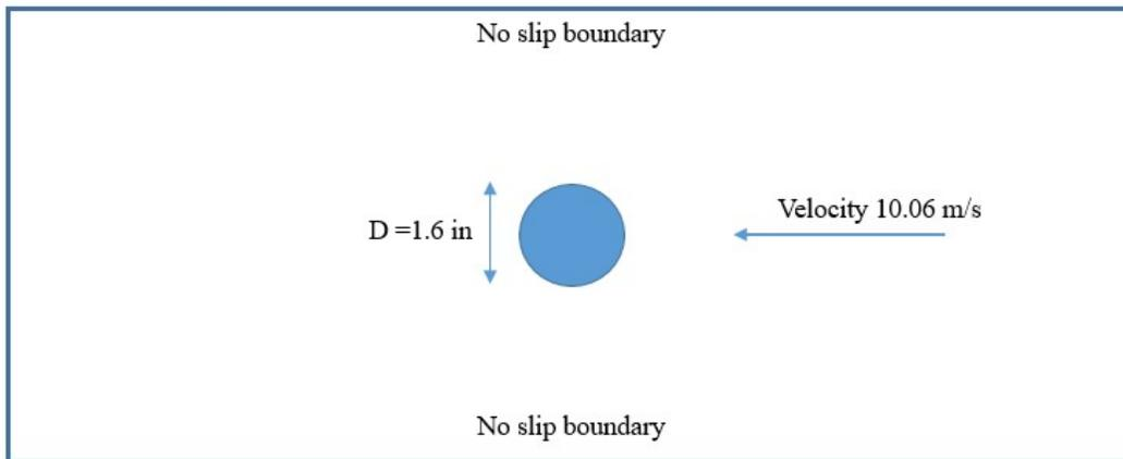
**Figure 5.** The Physical Model for the Cylinder
