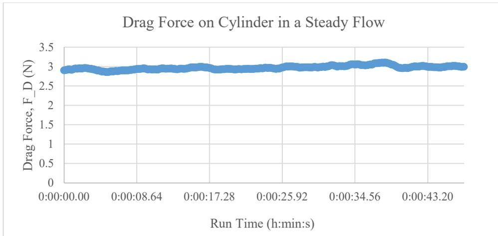
**Figure 11.** Drag Force on the Cylinder over Time
