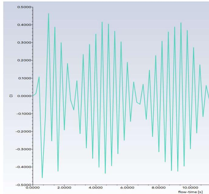
**Figure 8.** Coefficient of Lift for the Cylinder in ANSYS over time
