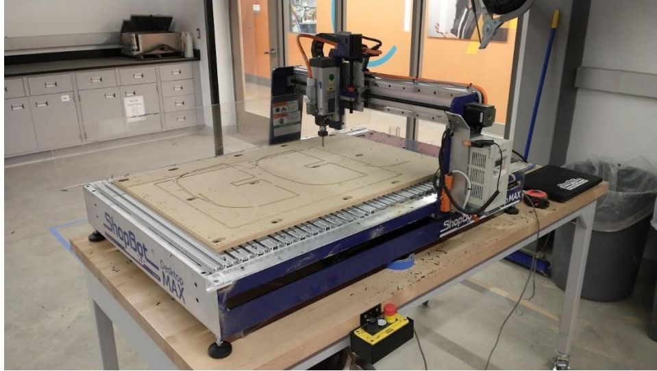
Figure 1: Models were cut using a ShopBot D364 Desktop MAX router [9].
