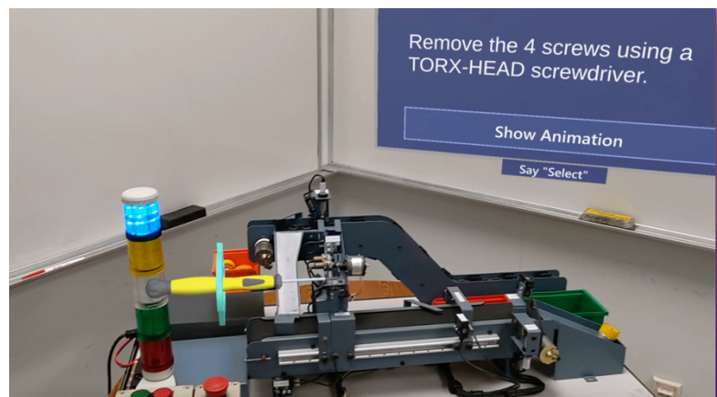
Figure 7: A simpler IAU that has a textbox and an animation of a virtual screwdriver.
