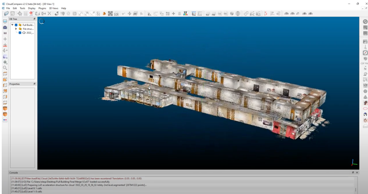
Figure 7. Demonstration of the entire building in CloudCompare software tool.
