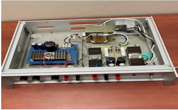
Figure 3: Student power supply enclosure design: example 2
