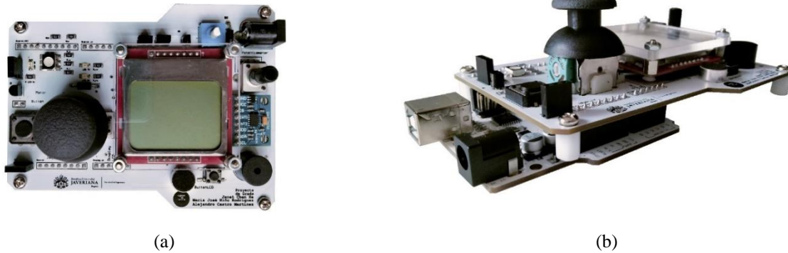
Figure 3: (a) Shield implemented (b) shield coupled with an Arduino UNO
