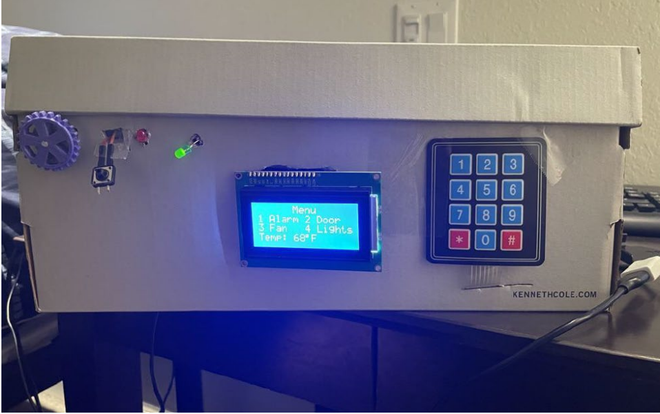
Fig. 5 smart home system designed by one of the student groups
