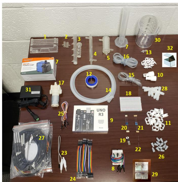
Figure 3 – Actual picture of kit components (left) along with list and nomenclature (right) used in Figure 2.
