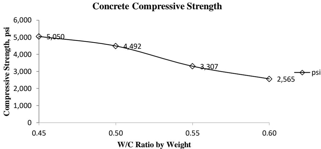
Figure 7. Compressive strength graph by water cement ratio
