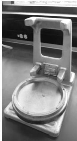
*Figure 4.* Capping mold
