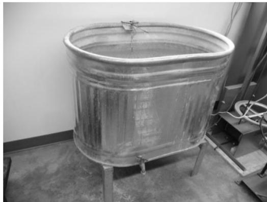
*Figure 2.* Concrete cylinder curing tank
