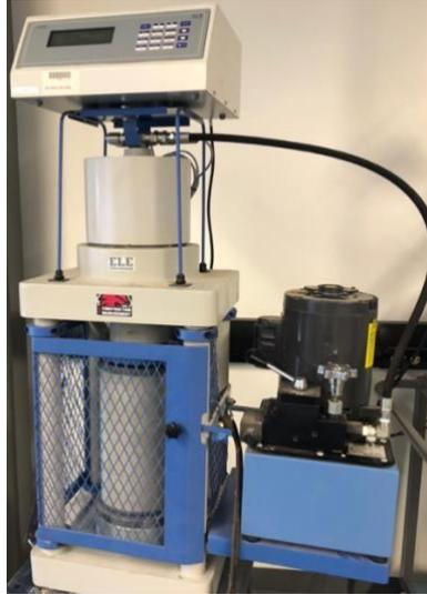
Figure 5. Digital Concrete compression tester with readout
