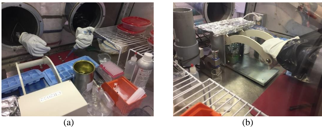
Figure 5: Assembling cells (a), and crimping to sealed cell (b).
