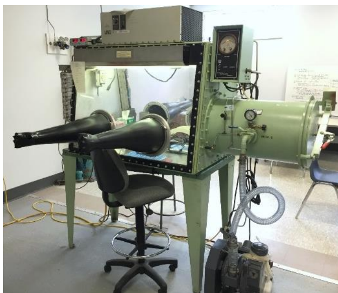
Figure 4: The LTU glovebox with vacuum pump in the lower right of the photo.
