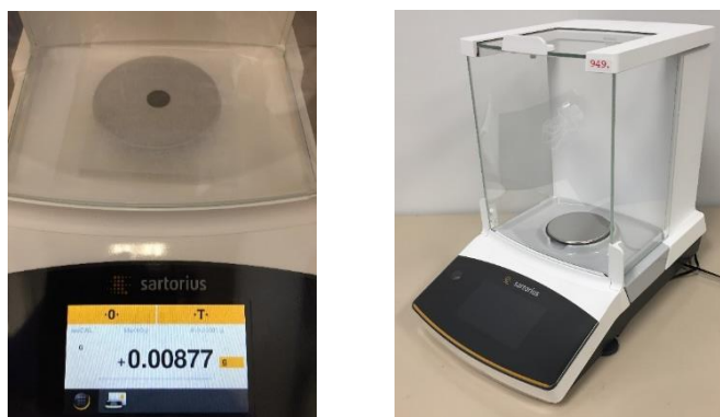
(a) (b) Figure 3: An electrode disk weighed (a), and the balance used (b).
