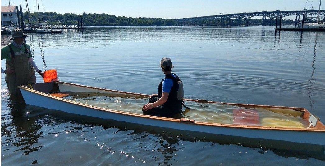
Figure 13. Sea trials: the swamping test. The goal was to see if the boat was stable with one-person while swamped. While it was, the reserve buoyancy was insufficient to pass USCG standards for commercial construction, a known design feature. The skiff built the previous year was designed to meet the standards and the students saw first-hand the difference built-in buoyancy provides.
