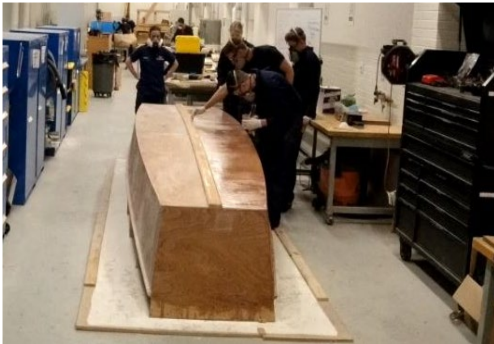
Figure 10. Fiberglassing the bottom of the boat with one layer of 6-ounce boat cloth.
