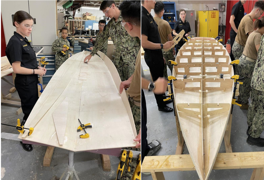
Figures 1 and 2. Stitching the bottom and side panels together (left) and assembling the internal frames (right) in the fishing paddleboards.
