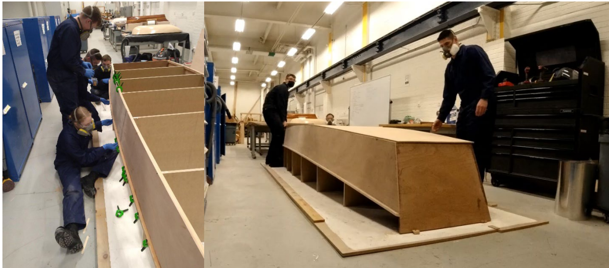
Figures 8 and 9. Gluing on the gunwales (left) and dry fitting the bottom (right).
