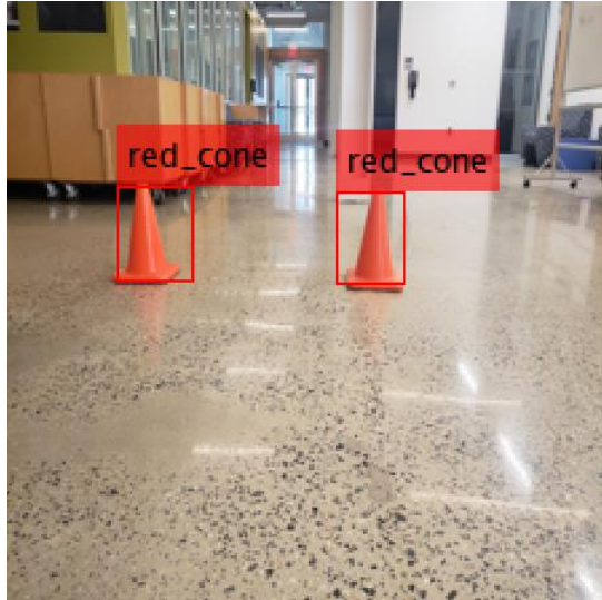
Figure 3: Traffic cone detection with Yolo object detection algorithm
