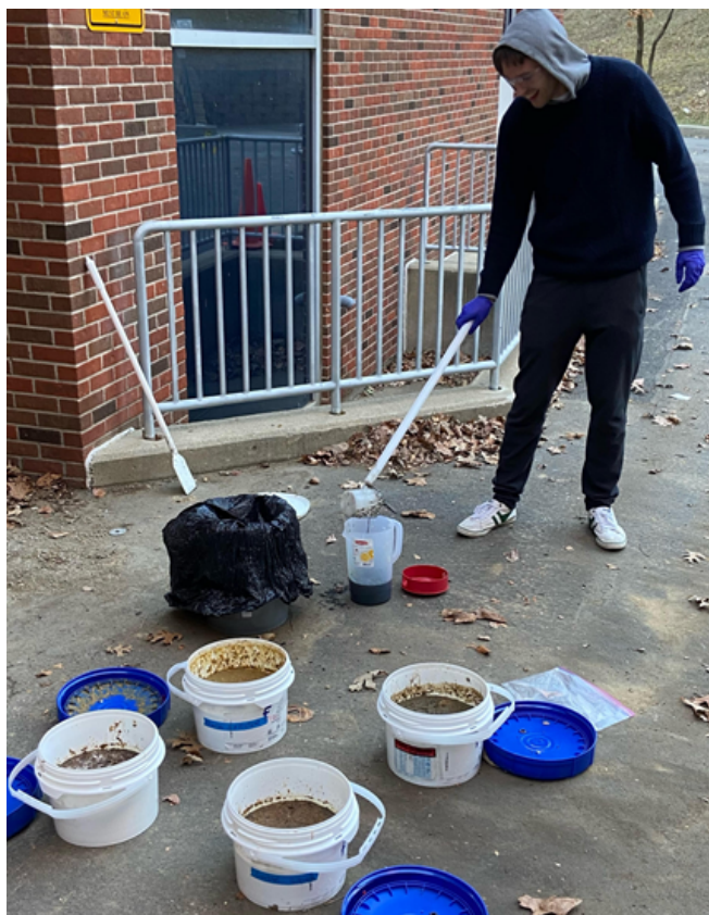
Figure 1. A ChE student adding inoculant obtained from a local water treatment plant to be blended with organic residues prior to sealing the biodigesters [Photo provided by a student].
