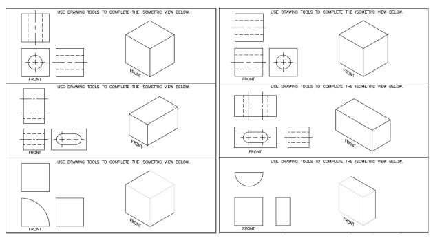
As illustrated in Figure 3, the first question of both assessment versions was a cube with a circular hole in one plane, similar to one shown in the instruction. The second and third questions were transfer items to different shapes. Question 2 required drawing two ellipses, and Question 3 required relating the drawing of isometric holes to rounded external surfaces of objects.
