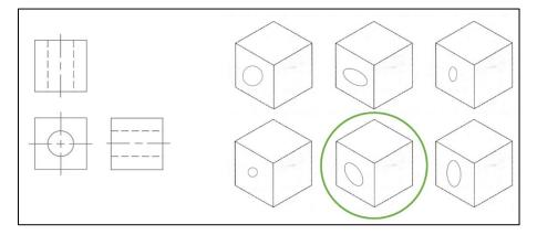
In Part 2, students were given a handout with a two-dimensional multiview of a different object and were instructed to draw the holes in the isometric view (see Figure 2). Students were provided multiple (identical) isometric views to explore various techniques for drawing the holes depicted in the two-dimensional multiview.
