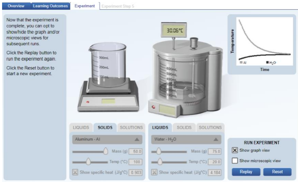
Fig.4 Home-based Virtual Lab Set Up for Specific Heat of Solids
