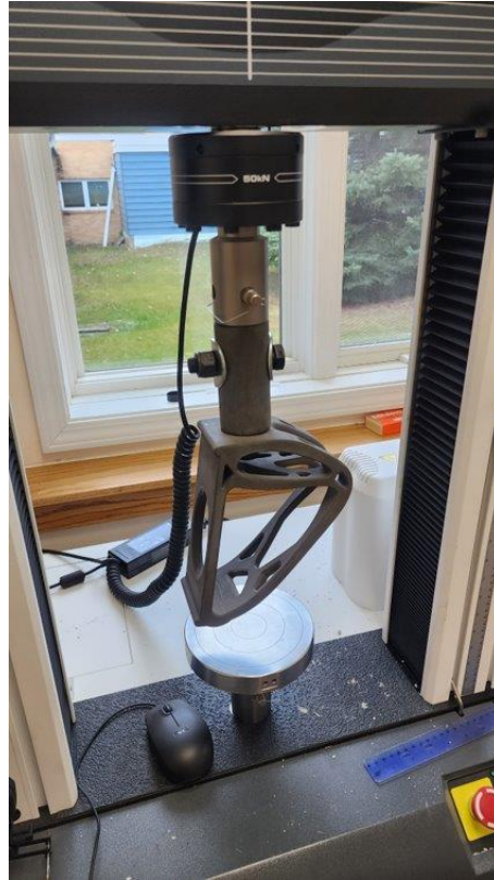
Fig. 3. The image shows the prosthetic device affixed to the personalized bracket used for compression tests. These assessments not only validated the chosen material but also assessed the leg's construction. The findings gathered were utilized to evaluate the correlation between the real-world dynamic tests and software stress simulations.
