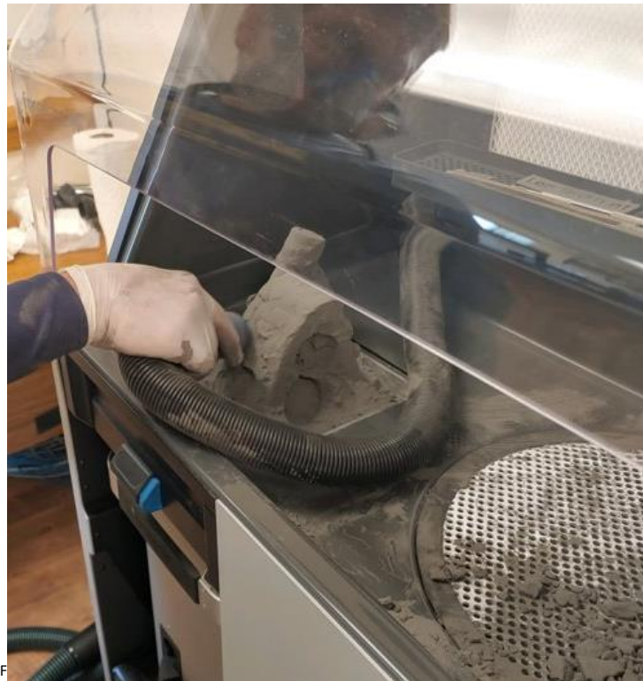
Fig. 1. Pictured above is Laboratory-technician tribal-engineering student unpacking the powder-block, post fabrication. The un-sintered, loose material will be collected, sifted, and recycled for use on future projects. This is all done inside a negative airflow hood that filters out particulates, keeping the technicians safe.
