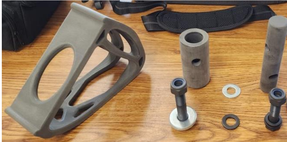
Fig. 4. In this image, we can observe the latest prosthetic leg design undergoing post-processing, along with a specially-made mounting jig for conducting dynamic real-world testing. The connecting sleeve at the center increases the diameter of the prosthetic, allowing for more accurate force transfer to the stanchion arm above and ensuring precise load cell readings. The nuts and bolts visible in the picture serve only as keys to align the various components and are not structurally significant. Finally, the post on the right is designed to fit into the 50 kilonewton load cell of the testing apparatus.
