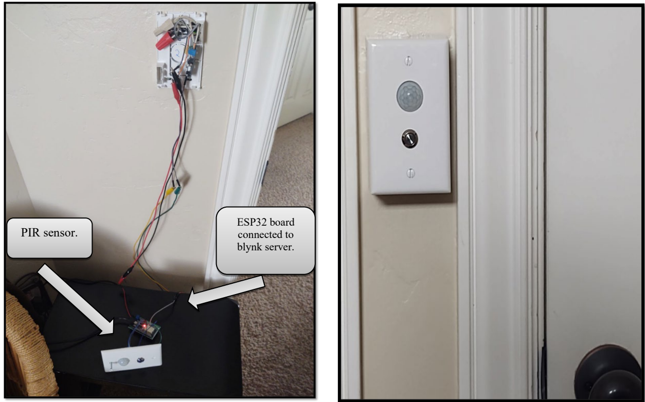
Figure1: Node in the Bedroom – One ESP32 Wirelessly Connected to the Sensor Network [16]
