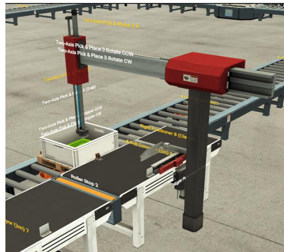
Figure 9: pick and place the product in the box by using the handling machine
