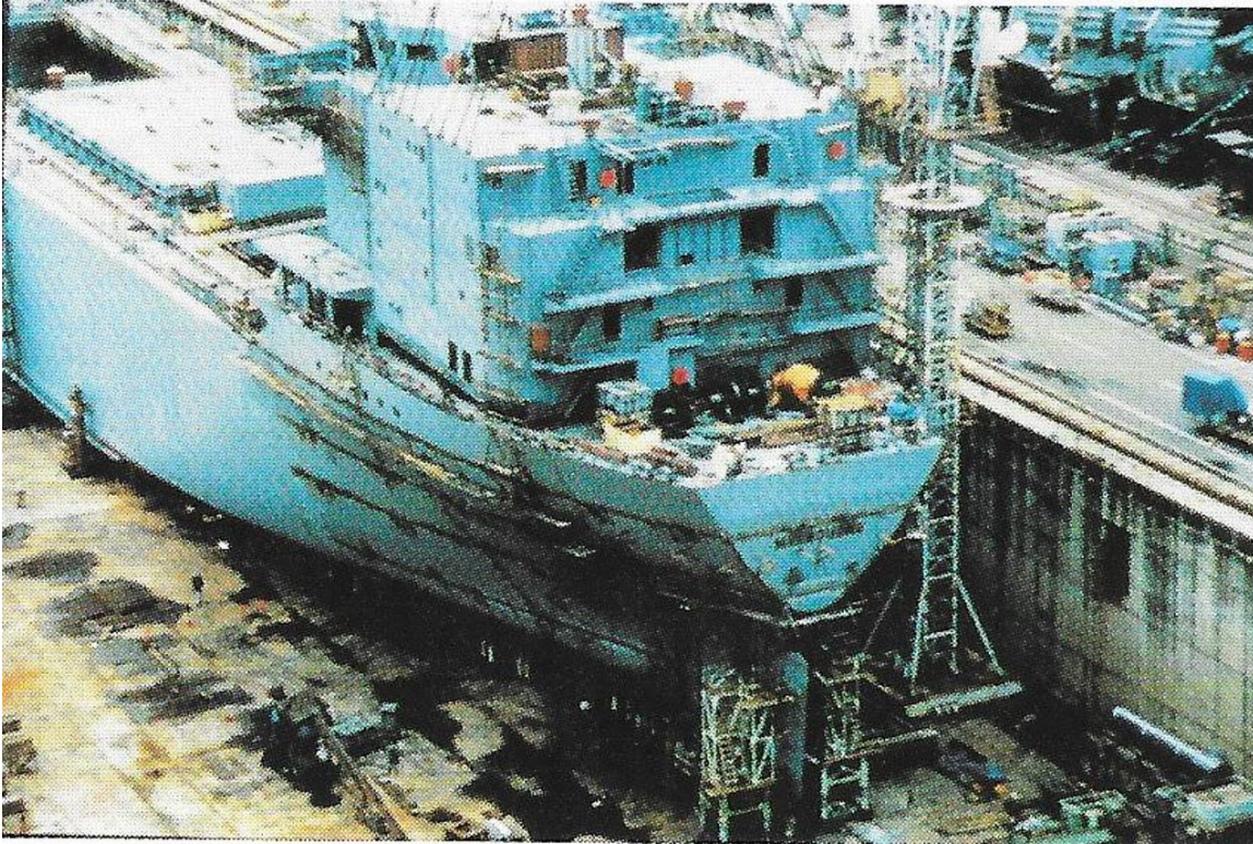
Figure 6 – Insertion of the After Deckhouse Module (or Unit or Block) [12]
