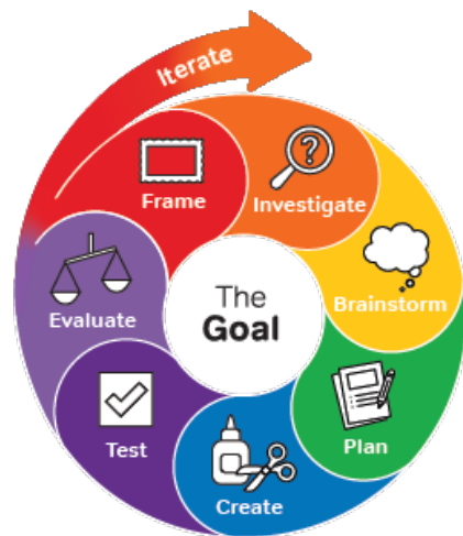
Figure 2: YES Middle School Engineering Design Process
