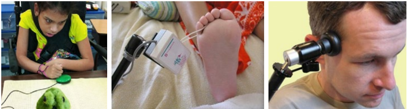
Figure 5: Alternative activation switch examples. Alternative activation switches plug into the female jack on an adapted toy. This allows the toys to be activated by pushing a nearby large button (left), moving a toe (middle), or tilting one's head (right.) Images (from left to right) from Ablenet, Patycare.org, and Enablemart.
