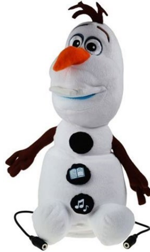
Figure 4: Adaptable toy example. This Olaf plush toy is normally activated by pushing the small buttons on his chest. The adapted version (shown here) has added universal female jacks for alternative activation switches. Image from Desktop Technology Services Limited
