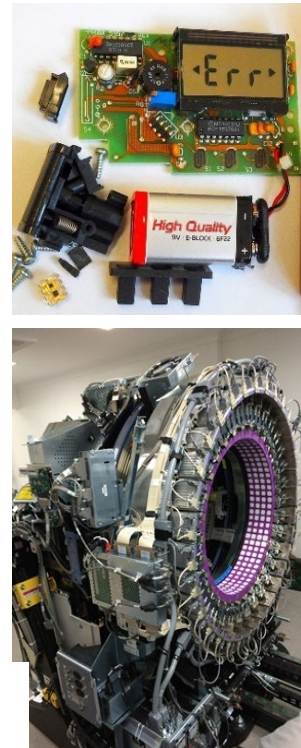
Figure 1: Circuits in medical devices. Circuits are used to power small, patient-used medical devices such as glucose meters (top) as well as large, hospital equipment such as computed tomography scanners (bottom.) Images (from top to bottom) from DiodeGoneWild and Meditec
