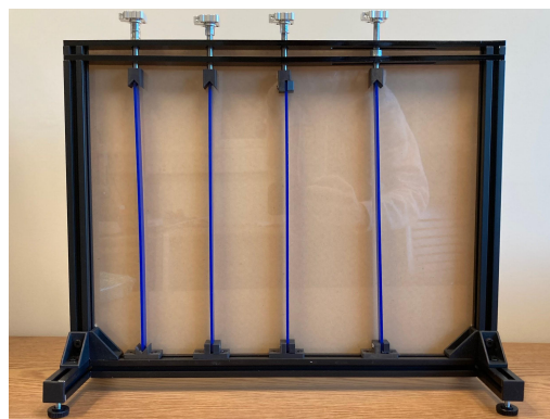
Figure 4: Picture of the Euler buckling model (Constraint conditions from left to right: pin-pin, pin-fixed, fixed-fixed, free end- fixed)
