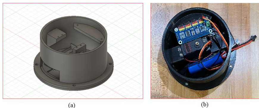
Figure 1. Base of the Robotic Arm (a) 3D CAD Model; (b) Base with Hardware
