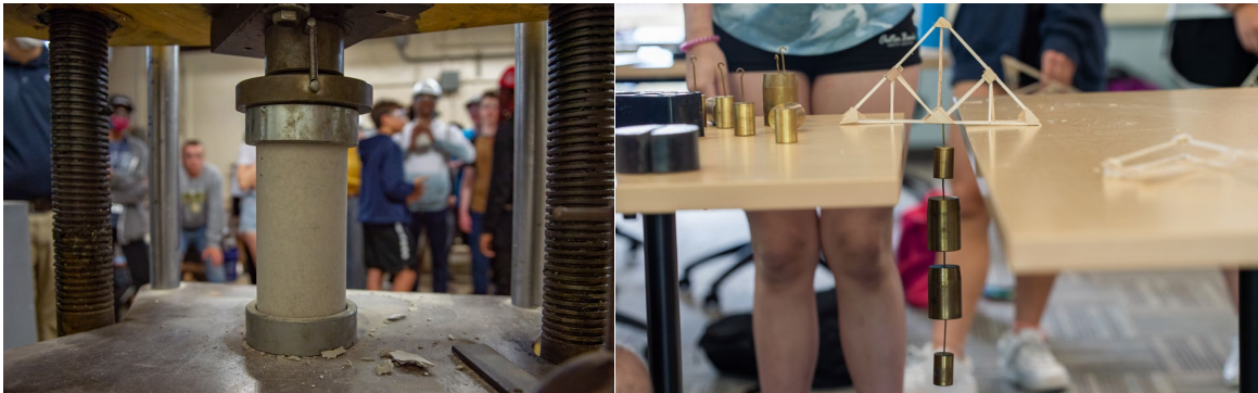
a) Loading a concrete cylinder specimen b) loading a balsa wood truss.
