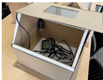
Figure 3: Example set up of the insulated mini house experiment.
