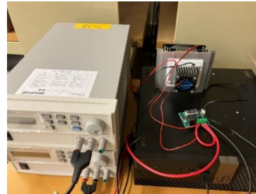
b) Demo 3 peltier cooling with a temperature controller
